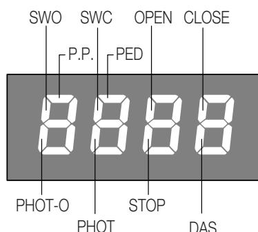
N.C. inputs are represented by the vertical segments. N.O. inputs are represented by the horizontal segments.
